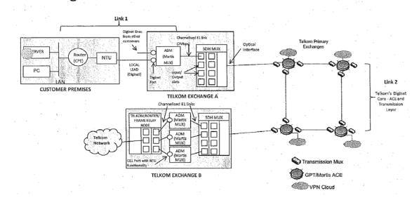
Diagram of Telkom access links to its own networks
